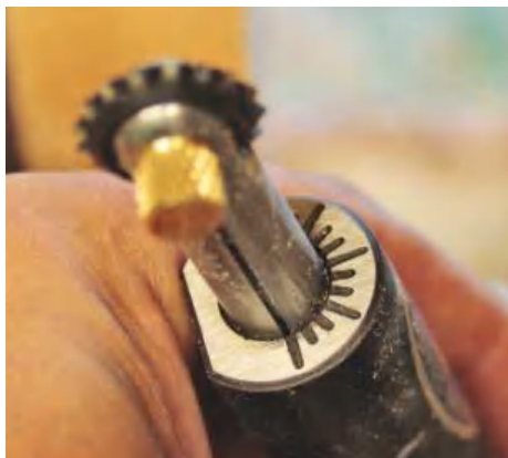
▲ The sleeve rotates to register against the cursor mark on the tool shaft
